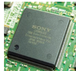
The graphic chip that was used to calculate all of the polygons used in PlayStation games. Without it, the 32-bit titles would have been flat. As a side note it is as efficient as managing both 2D and 3D.
